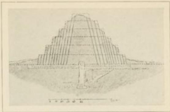
FIG. 71. — COUPE DE LA PYRAMIDE A DEGRÉS.
