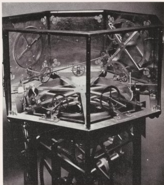
FIG. 44. Modern reconstruction from manuscript descriptions of the astronomical clock of Giovanni de Dondi, ca. 1364. Note the equilateral triangular teeth which survived in even later clockwork in spite of their inefficiency. Copyright Science Museum, London.
