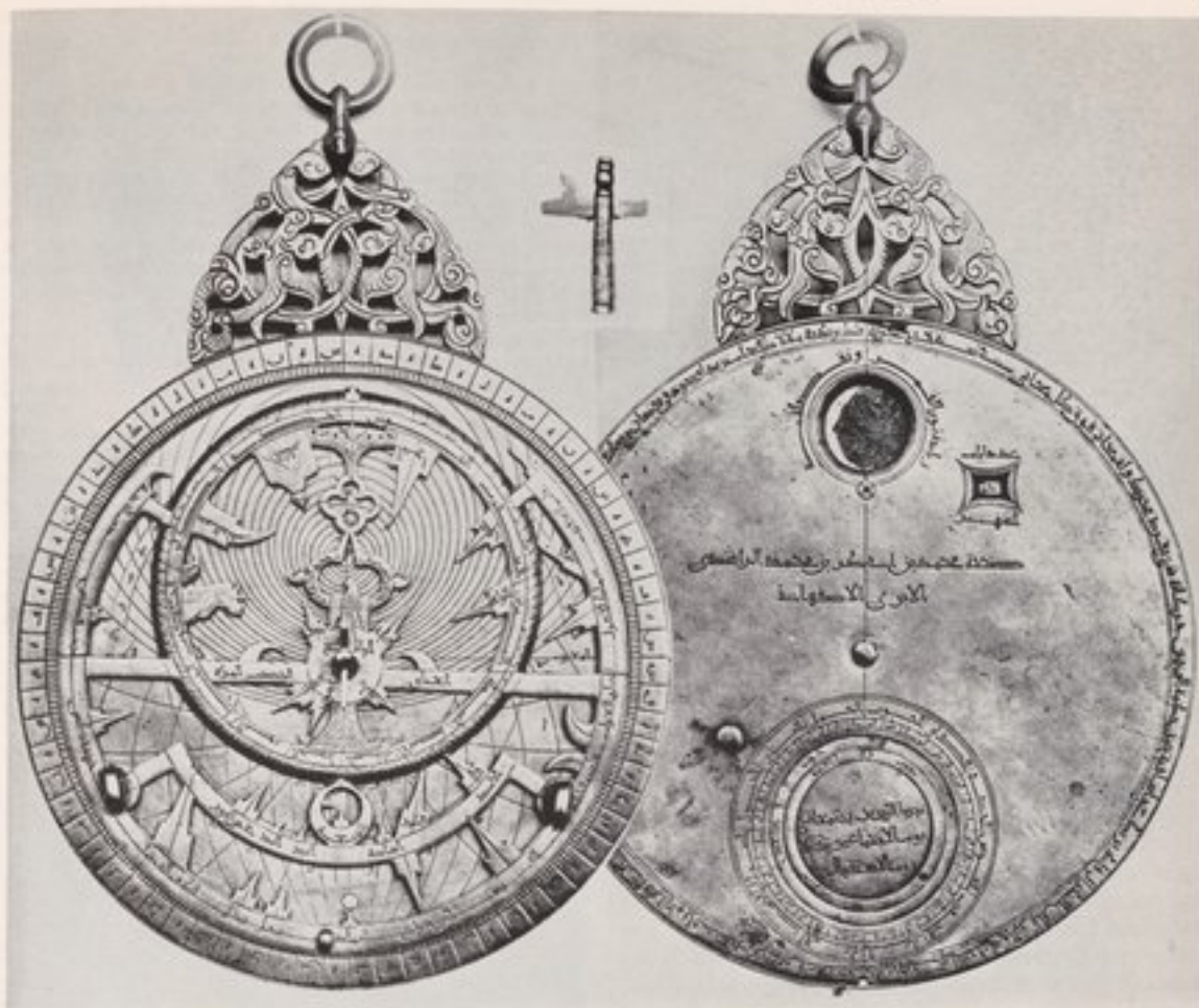
FIG. 42. Astrolabe containing geared calendar work. The instrument, now in the Museum for History of Science, Oxford, was made by M. b. Abi Bakr, Isfahan in 1221/2 A.D. and the gearing follows the design reported by al-Biruni ca. 1000 A.D. and contains many similar features to the Antikythera mechanism.
