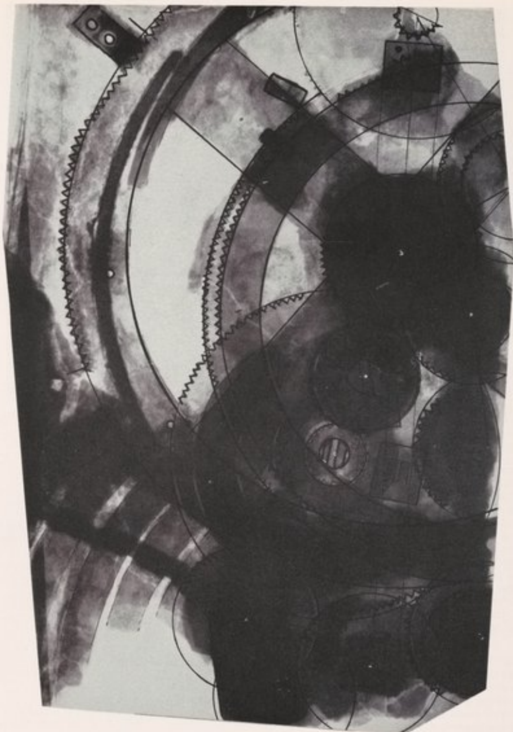
FIG. 23. Sample of alignment radiographs showing teeth, wheel circles, axes, etc., marked in ink for tracing the gear trains.
