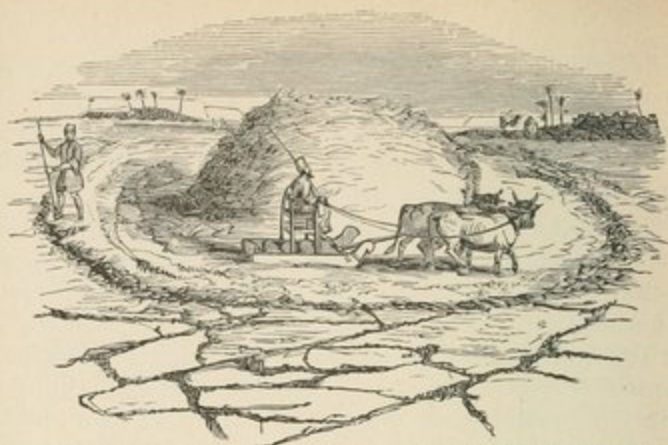
VIGNETTE F. — The Noreg, a machine used by the modern Egyptians for threshing corn.
