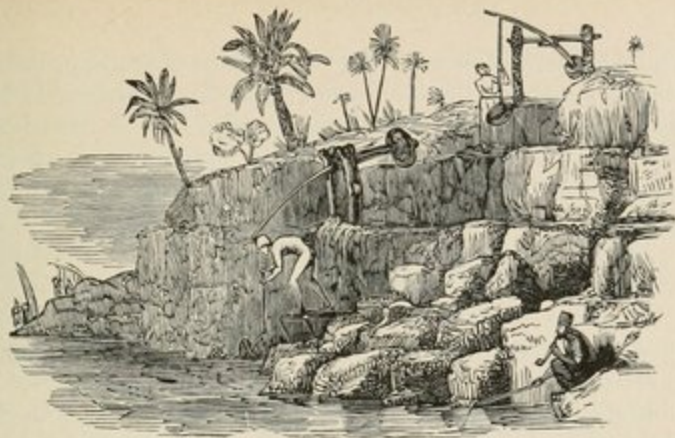
VIGNETTE D. — Modern shadoof, or pole and bucket, used for raising water, in Upper and Lower Egypt.
