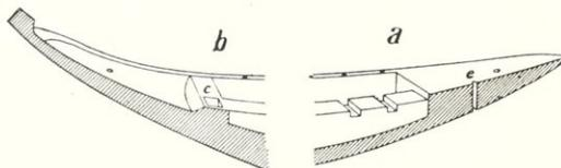
Fig. 21. — Sections of bow and stern.
