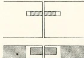
Fig. 316. — Holes for metal bond.
