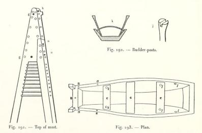
the back edges. In the first seat from stern two slanting posts (1) with slot in head (fig. 192). In the bow, side of boat is pierced by hole on each side (1, fig. 193).
