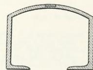
Fig. 287. — Elbow beam of k-n, vestibule.
