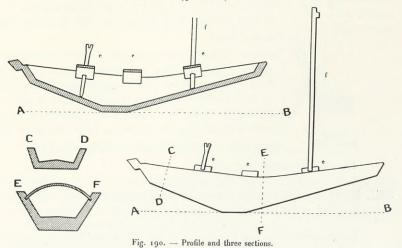
HULL: Broad flat boat with bow and stern square cut. Stern has small projection (fig. 190)
