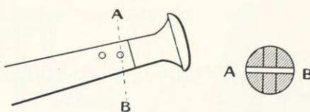
Fig. 58. — Slot joint on bow.
