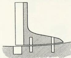
Fig. 72. — Mast-shoe, section.
