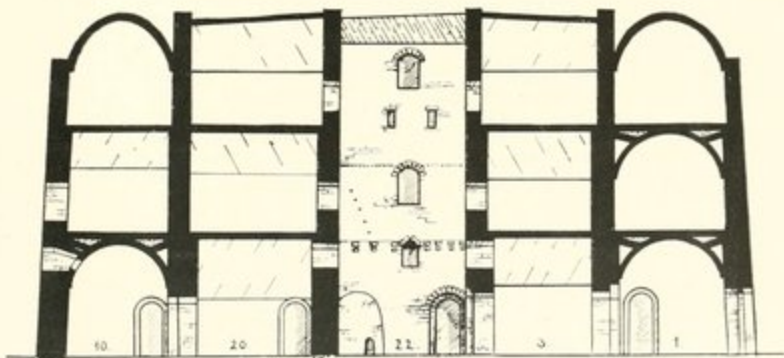
Restored section East by West along line B . . . . . B in ground plan, Pl. 21.
