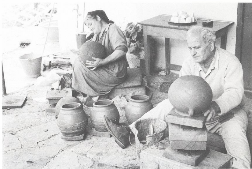
Fig. 3.1 Traditional potters shaping cooking pots first shape flat-bottomed forms whose rims and upper bodies are completely finished and set aside to dry. Three cooking pots rest on squares of wood or bark as the clay dries slightly before handles are added. Strings wrapped around the lower bodies serve as an external support for the wet clay, functioning as a mould. When the rim is almost leatherhard, but the base is still wet, the potter (in the background) removes the strings and then scrapes away excess clay from the flat base to create a rounded bottom. Her husband then returns each cooking pot to the turntable (two are piled here on top of each other to increase the height and make the work easier) to smooth the surface by rubbing it with water and a bamboo tool (standing in the broken bucket). Halloumi cheese dries on a table in the background of this courtyard in Kornos, Cyprus, 1986. Photograph by G. London.
