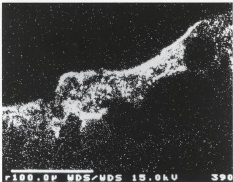
Plate 12: Tin x-ray map of Crucible MRN 537 cross-section. SIMS. Mieke Adriaens.
