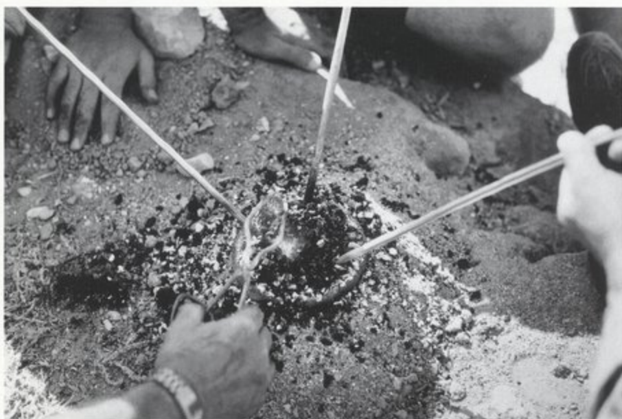
Plate 17: Experimental Smelt, Celaller Village using three blowpipes.
