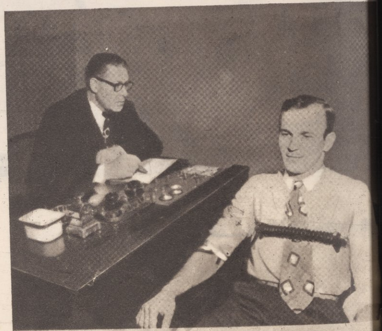
In ideal arrangement for deception tests. Note Polygraph mounted flush with top of table
